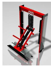
The launcher is a frame of aluminum tubing made to cradle the ball. The bottom is attached to a hinge, and the top to surgical tubing. When under tension, this tubing pulls the launcher upward, propelling the ball (hopefully) into the goal.
