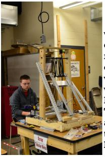
In prototyping, we found that the catapult expended much of its launching energy to unwind the winch. To counter this, we added the torsion bar with a latch on it. This allows us to use all of the energy from the surgical tubing to launch the ball.
