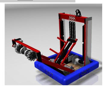
The catapult system consists of a complex series of mechanisms. In cooperation with the winch, detailed on page 7, the catapult consists of a launcher and a torsion bar.
