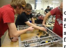
Apollo drives on the 2014 Drive-ina-Day Square Chassis from Vex Pro. This system offered us flexibility in terms of mounting and area.
