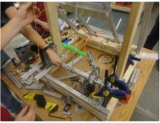
Once a ball is in range, the brake disengages and the winch primes to shoot. After priming, the brake reengages to prevent backdriving. Once we are ready to launch, the latch on the torsion bar releases. The winch then unwinds to return the torsion bar
