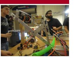
The assembly is deployed using pneumatic cylinders. The rollers are powered using a Bane-Bots 550 on a 16:1 planetary gearbox with a 15:54 open gearbox.
